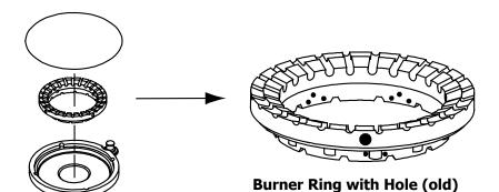
Does not work with new version of ignitor assembly.
