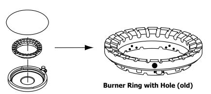
Does not work with new version of ignitor assembly.
